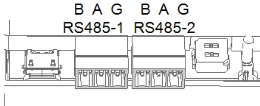
Figure 6: RS485 connectors and termination switches
