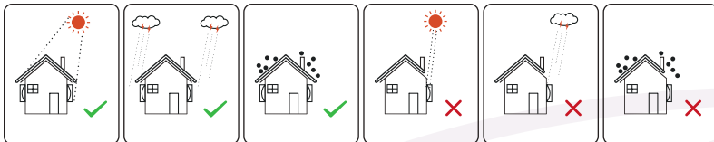
Figure 4-1 Recommended installation location
